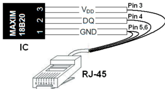
The cable of the detector can optionally be extended up to 50 meters with a network cable and a 2 x RJ45 adapter. (see pictures)
